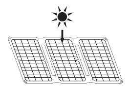
Position the solar panel in most direct angle towards the sun as possible.
