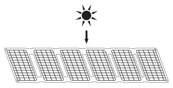
Position the solar panel in most direct angle towards the sun as possible.
